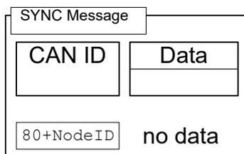
For SYNC operation, transmission mode (Transmission Type) 0 is normally used for the RX-PDOs (data are valid with the next SYNC); for TX-PDOs, a transmission mode between 1 and 240 is selected. (Details: see chapter Process Data Object (PDO)).
