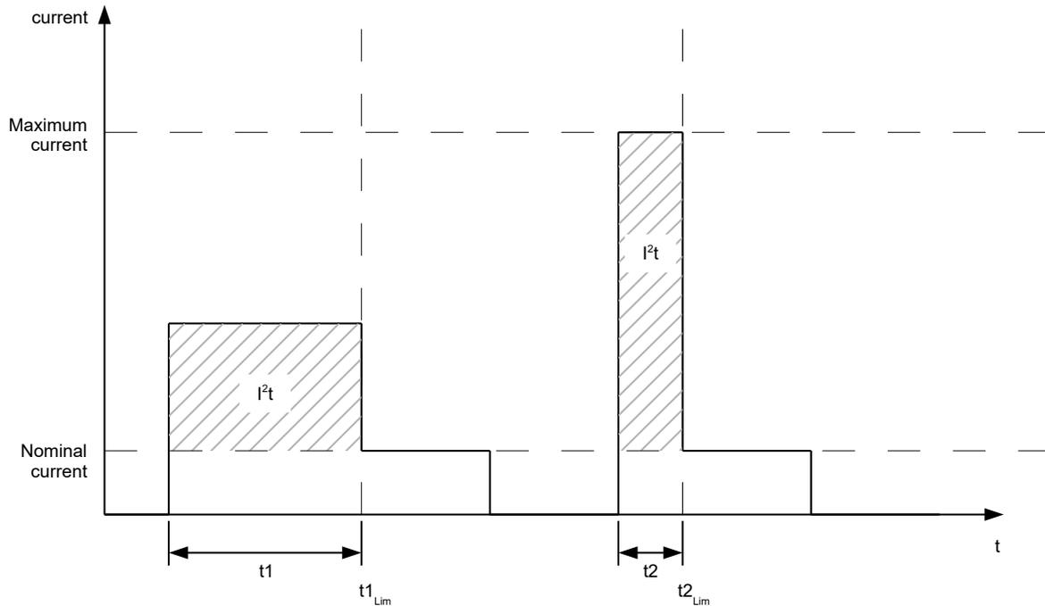
In the first section,  $t1$ , the current value is higher than the rated current. At time  $t1_{Lim}$ ,  $I^2t_{Lim}$  is reached and the current is limited to the rated current. A current that corresponds to the maximum current then occurs for a period of time  $t2$ . Hence, the value for  $I^2t_{Lim}$  is reached more quickly than in time  $t1$ .
