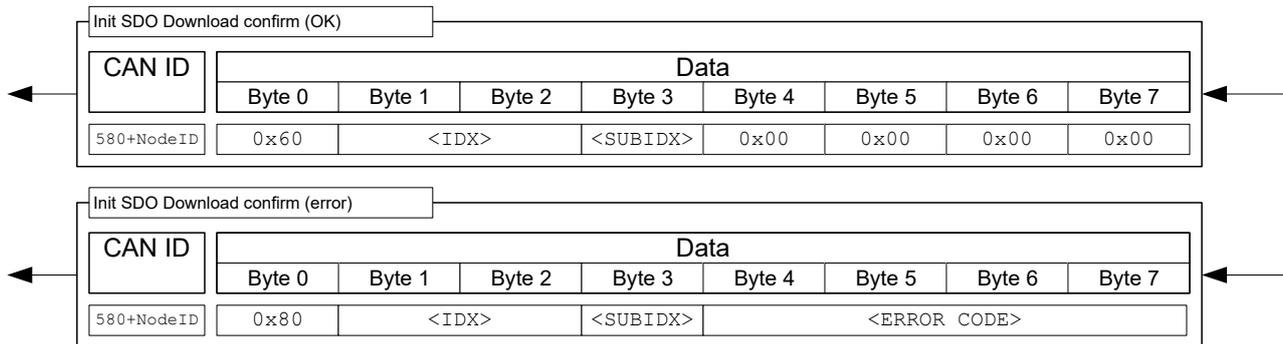
**Example:** Set object 607A<sub>h</sub>:00<sub>h</sub> (target position, SIGNED32) to value 3E8<sub>h</sub> (=1000<sub>d</sub>) of a controller with node-ID 3:
