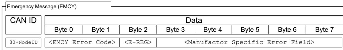
A total of three error codes are transferred here: the "Emergency Error Code" (<EMCY Error Code>), the content of the "Error Register" object (1001<sub>h</sub>, <E-REG>) and a manufacturer-specific code (Manufacturer Specific Error)
