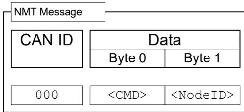
Here, the <CMD> corresponds to one of the following bytes (see also the legend in the figure of the NMT state diagram):
