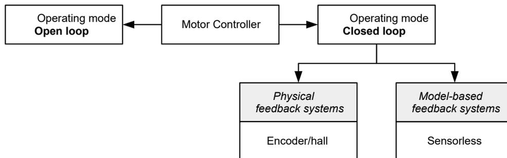
Summarized in the following are all possible combinations of control modes and feedback systems with respect to the motor technology. Support of the respective control mode and feedback is controller-specific and is described in chapters [Pin assignment](#) and [Operating modes](#).
