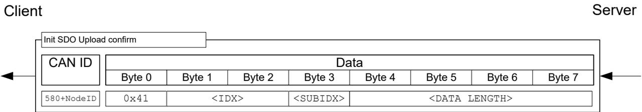
The initialization is thereby concluded; all that remains is the upload of the data. A data packet is requested with the following SDO request:
