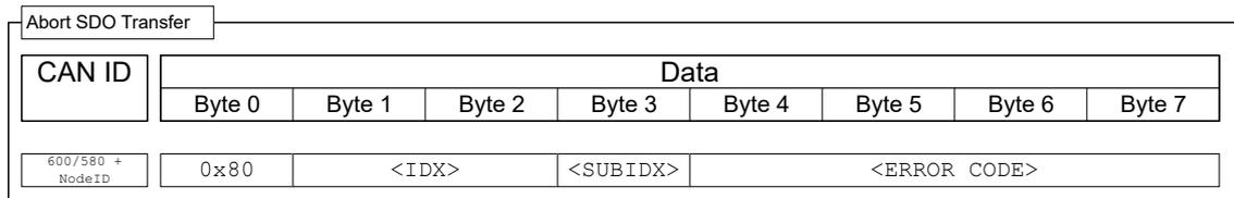
After receiving the message, the SDO transfer is considered ended; the service is *not* confirmed. A new SDO transfer must then be started from the very beginning. Transfer of the <ERROR CODE> is optional; the controller does not evaluate the code.
