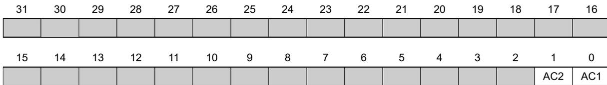
In general: If a bit is set to the value "0", the analog input measures the voltage; if the bit is set to the value "1", the current is measured.
