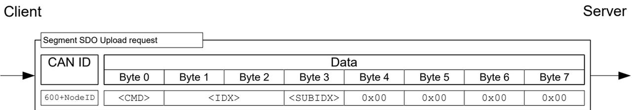
Byte 0 with command <CMD> is structured as follows:
