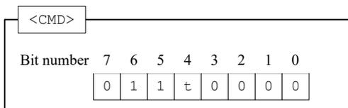
The bit with designation t alternates with each request ("toggle bit"). It begins each transfer with 0, even if the previous transfer was aborted.
