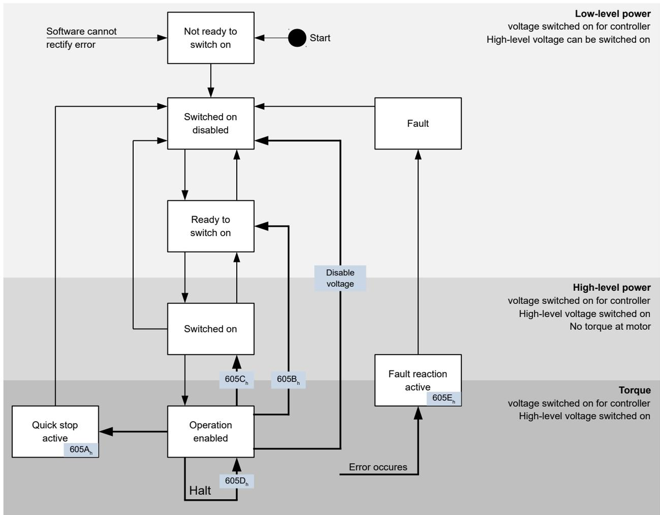
Transition with break reaction Index of the object that specifies the reaction
