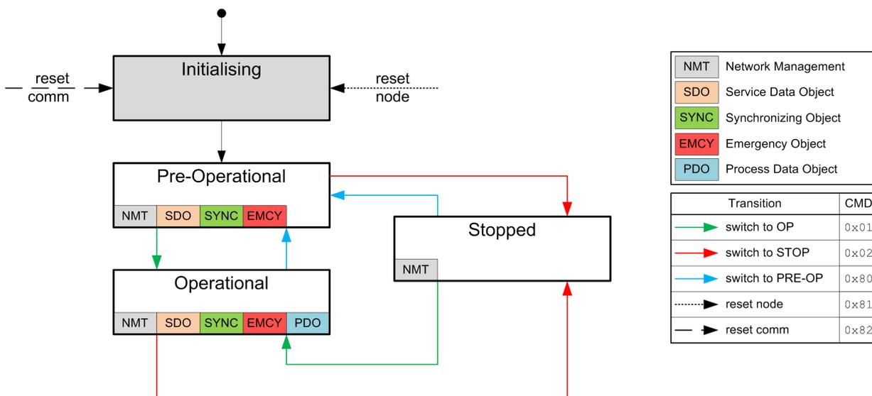
Shown in the following table is an overview of the activity of the services in the respective states. Note that the *Stopped* state stops communication completely and only permits controller of the NMT state machine.
